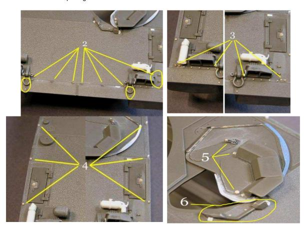
7. Right behind the driver hatch right side is welded a small bit of rod.
